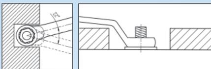
Deep-set bolt connections can be loosened optimally due to the offset ring heads and the ratchet mechanism.
