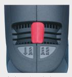
Clockwise/anti-clockwise switch on the top of the housing ensures maximum torque in both rotation directions via optimum positioning of the carbon brushes and extends the service life of the carbons.
