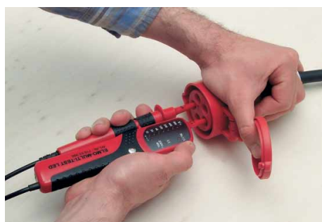
Phase sequence display (100 – 690 V). "One-hand" testing with spacer bracket.
