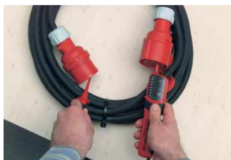
Conductivity test, optical and acoustic (0 – 500 kΩ).
