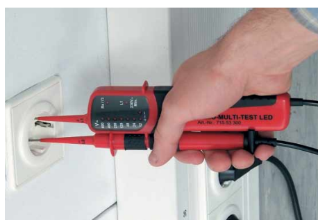
Voltage display with 7 LEDs (12 – 690 V). "One-hand" testing with spacer bracket. For voltages above 48 V, flashing display for safety. Automatic detection of direct and alternating voltage.
