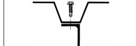
Galvanized drilling screws may only be used where dampness is not to be expected. For fasteners with construction approval, the approval and in particular Part 2 "Special regulations", must always be observed.
