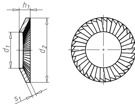
**Spring steel, mechanically galvanised, blue passivated**
