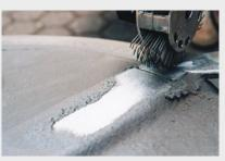
Removal of underbody seal and sealing compounds, and quick removal of paint.
