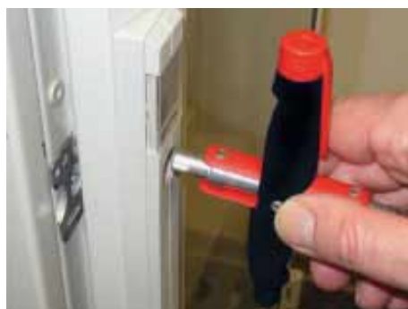
Double bit for switch box locks.
