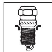
For conical sealing
