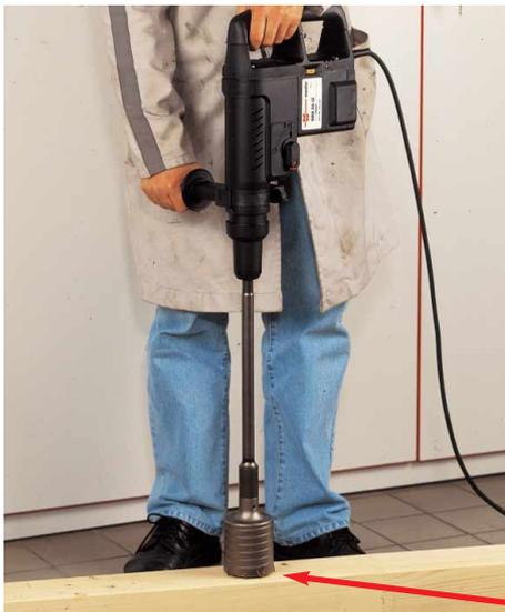
Simple release of adapter without additional tools with „striking impact“ on wood (set hammer drill to chiselling setting).
