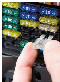
Remove existing flat blade fuse from fuse socket
