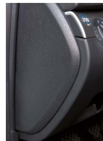
Closed fuse box
