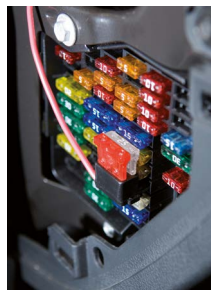
Plug flat blade fuse holder into existing fuse socket
