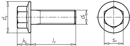
**MBN 10105, steel 10.9, with fine thread from M12. Silver-coloured zinc flake coating in accordance with DBL 9440.40 (form C  $\triangleq$  partial thread).**
