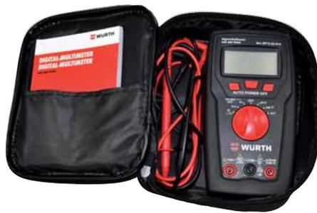
Modern, digital multimeter with effective value measurement (TRMS), cable break detector and LED pocket torch for professional use in trade and industry.
