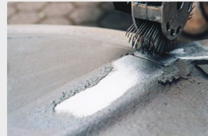
Removal of underbody seal and sealing compounds, and quick removal of paint.
