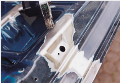
Paint removal in contoured and sharp-edged areas, 90° angle. No sand blast effect.
