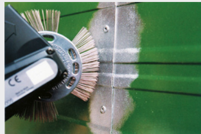
Removal of paint and corrosion from aluminium vehicle bodywork and assemblies, especially for rivets on truck bodies. No sand blasting effect!
