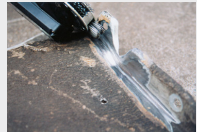
Especially suitable for applications involving weld seams, contours and edges. With sand blasting effect, ensures good adhesion for tin coating and trowel application.
