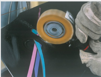
Removal of films, stickers and adhesive residues from metallic and paint surfaces. Contact surface twice as large ( w = 30 \text{ mm} ) as that of a conventional film rubber. Significantly faster material removal due to this and the increased rotation speed.
