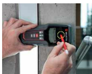
Locating iron reinforcements
