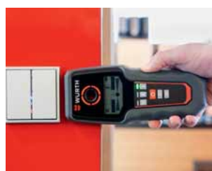
Locating energized and deenergized lines
