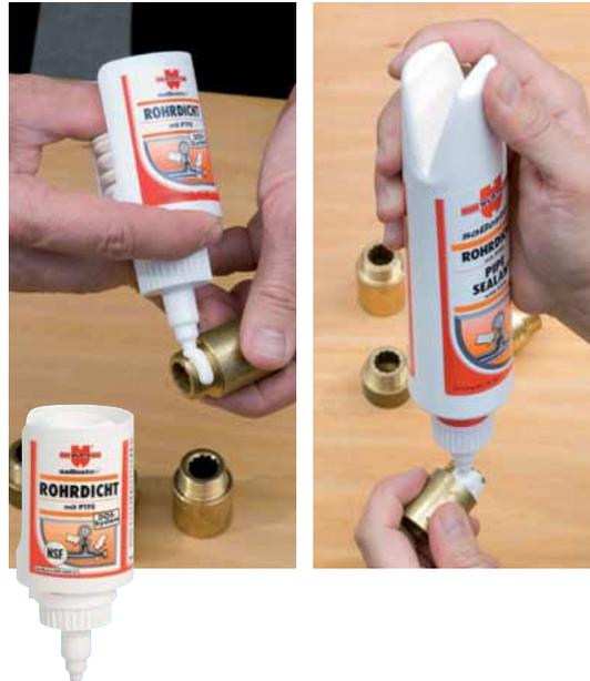
**For sealing all metallic pipe couplings and fittings with conical/cylindrical threads in accordance with DIN 2999**
