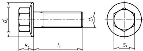
**MBN 10105, steel 10.9, with fine thread from M12. Silver-coloured zinc flake coating in accordance with DBL 9440.40 (form C  $\triangleq$  partial thread).**
