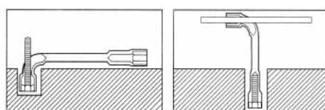
Specific offset and drill hole: A threaded rod or a lever pin can be inserted through. Thanks to the deep hollow design of the socket wrench, tightening is also possible with protruding threads.
