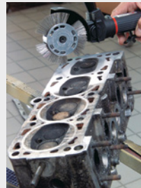
Removal of seals from grey cast iron. Not for Al or die-cast aluminium!
